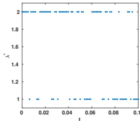
Parameter  $\lambda^*$  that maximises the nonlinear generator  $G$  over the noise coefficient  $\lambda \in [1, 2]$ .
